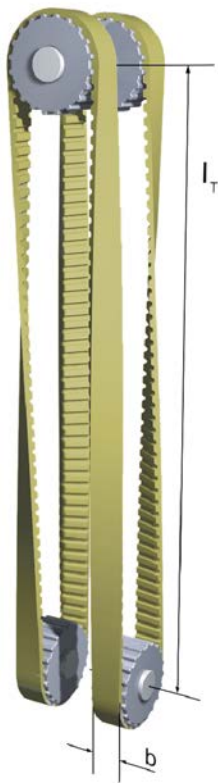
Angular drive with 2 axes
